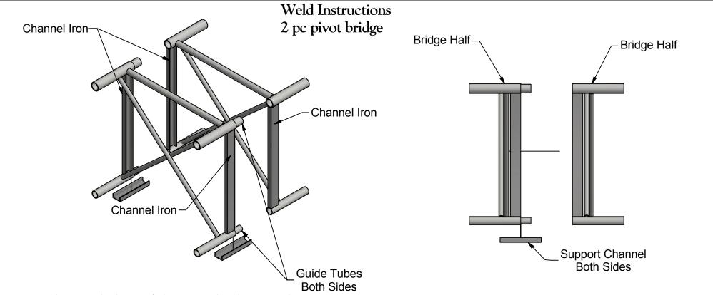
To join the two halves of the pivot bridge together.
