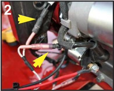
Disconnect the "Kill" wire from the wires leading from the yellow remote receiver box to the motor.
