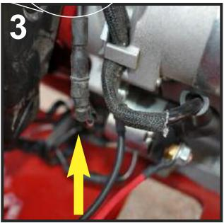
Connect the kill wires that lead directly to and from the Honda motor.
