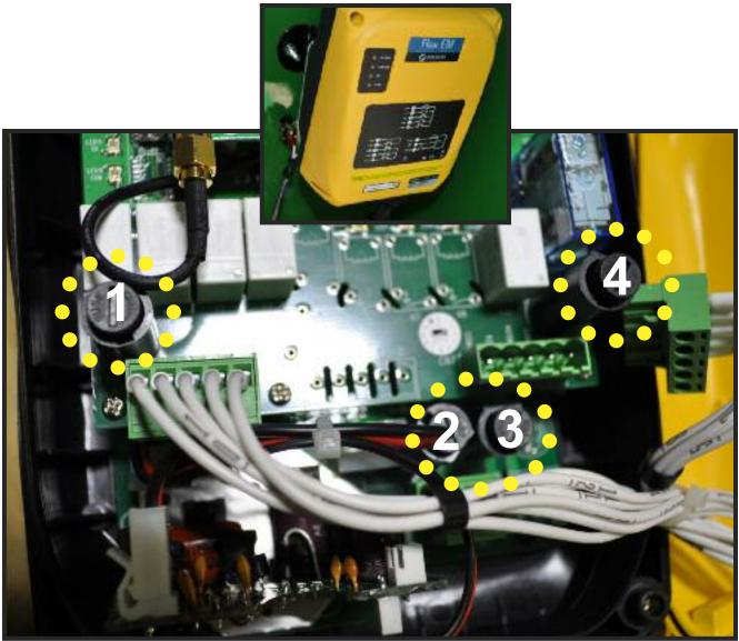
Using an ohmmeter, determine if the fuses are in working condition or not. If not, there are replacement fuses included in the owners' manual canister attached to the seed tender.
