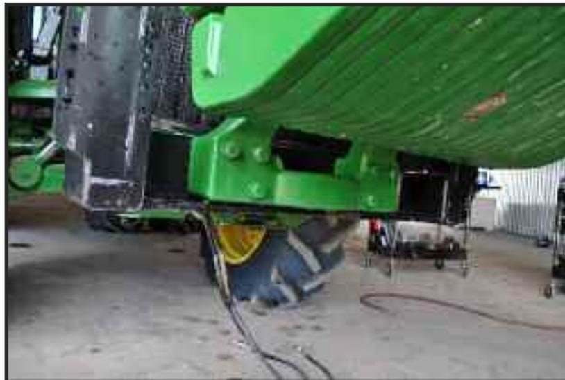
Step 4: Attach both the left and right side Height Adjustment Bar (Item 4 ) using provided u-bolts and nuts. Begin with bottom of the Height Adjustment Bar at 21" from ground.
