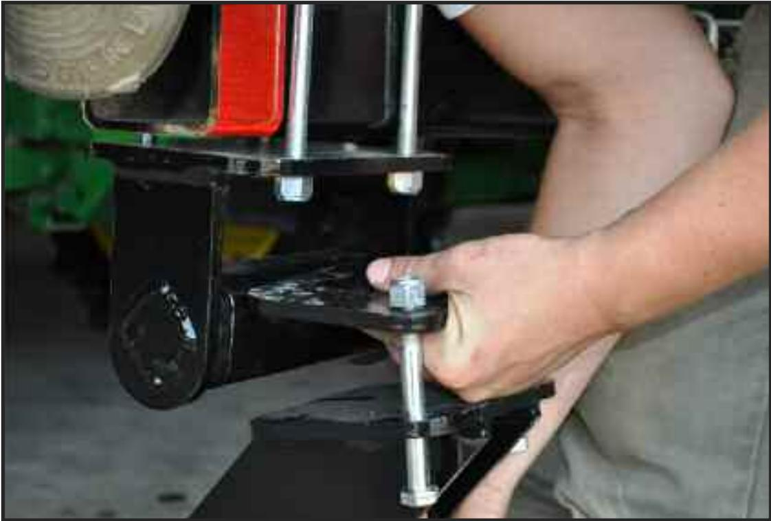
Step 14: Bolt two rear bolts to torsion shoe attachment plates as shown below.
