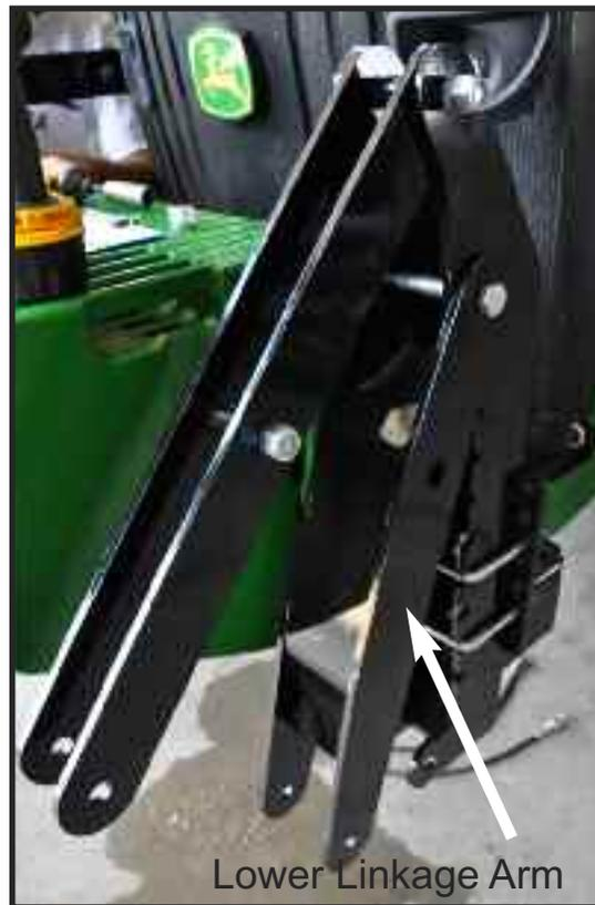
Step 7: Place Tool Bar (15) in front of tractor. Measure to find and mark the center. Measure distance between each height adjustment bar and note. Align square tube center with middle distance between height adjustment bars.
