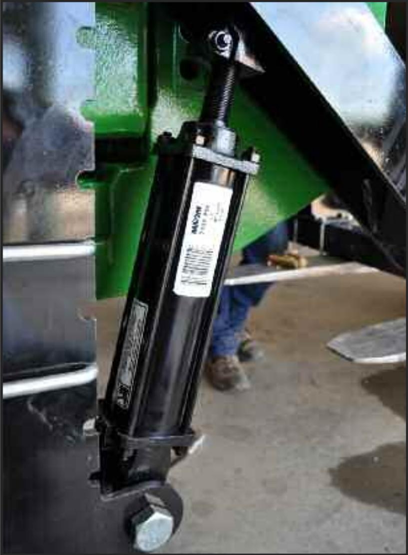
Step 11: Align lower linkage bar (7) with bottom bolt hole of lower linkage arm (13) and attach.
