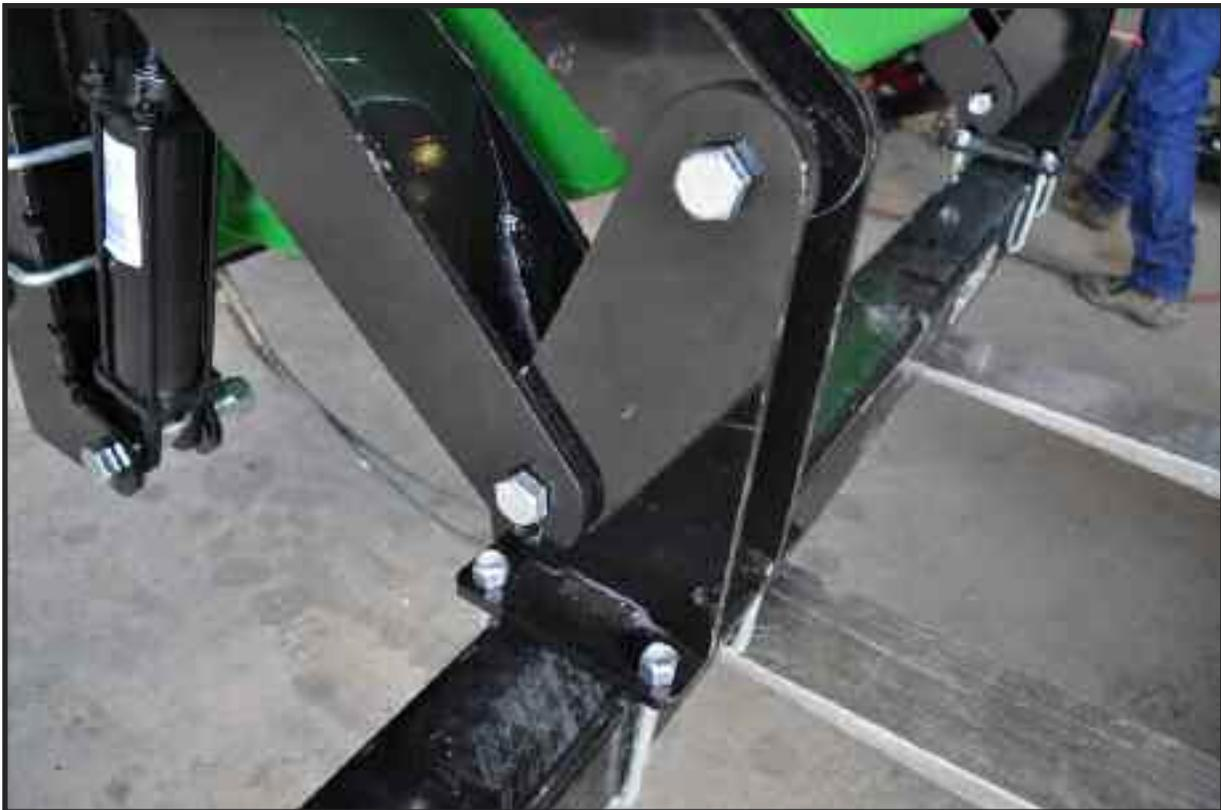
Step 12: Attach torsion springs (17) to tool bar (15), making sure they are aligned with the tractor tires.
