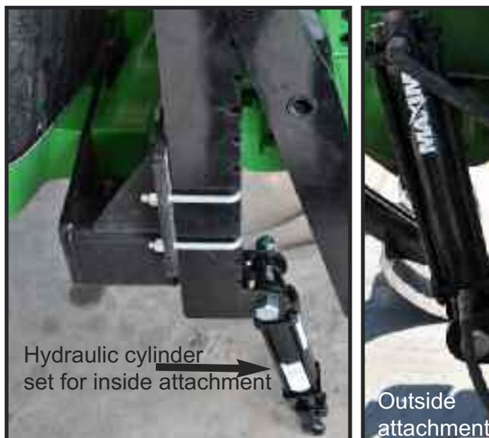
Step 9: Attach hydraulic cylinder with 1" x 5 1/2" bolts to lower linkage arm (13).
