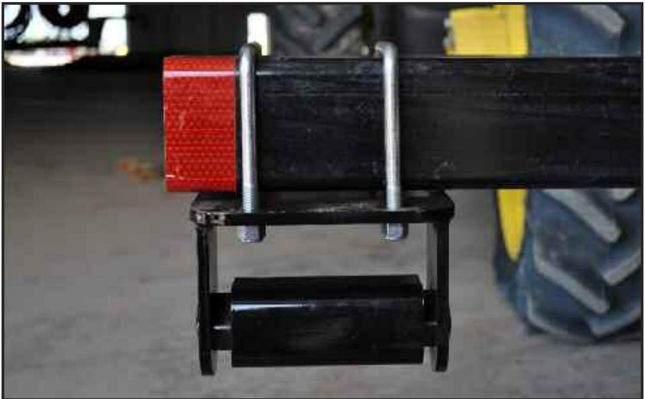
Step 13: Place two bolts in front bolt holes on torsion shoe attachment plates (18).
