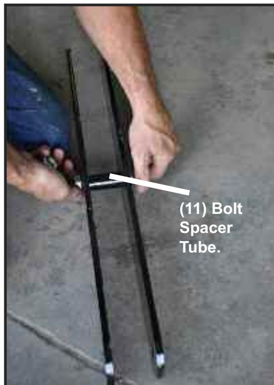
Step 6: Bolt linkage bars to height adjustment bars and attach Lower Linkage Arm (13) to Height Adjustment Bar (4).
