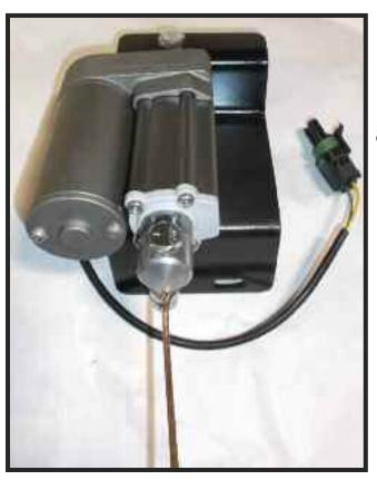
Place the 1/4" X 1 1/4" bolt through the hole on the actuator ram. Place 1 qty. 1/4" nut on the bolt and tighten. Next, place the throttle rod on the bolt and use 2 qty. 1/4" nuts on the bolt and tighten. The nuts will lock together and keep the throttle rod in place.
