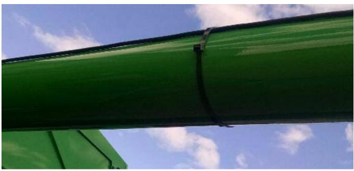
Use a heavy duty tie strap and attach the straight cable midway down the upper auger tube. Trim the cable tie. See above photo.
