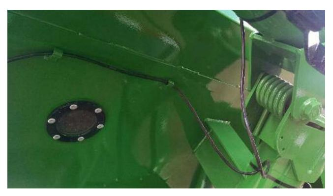
Locate the cable tabs on the seed tender body. Place the straight cable in these tabs and bend the tab over to retain the cable. Repeat with all tabs on the seed tender body.
