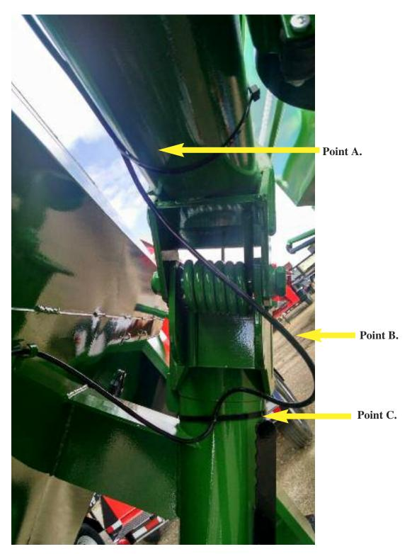
Attach the straight cable to the bottom of the upper auger tube (Point A). Leave some slack in the cable around the hinge area so the auger can fold without stretching the straight cable (Point B). Next, attach the straight cable to the top of the lower auger tube with a heavy duty cable tie (Point C). Finally, trim all cable ties.
