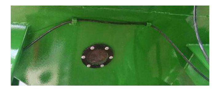
Locate the cable tabs on the inside of the front left leg of the seed tender. Transition the straight cable from the seed tender body to the seed tender leg.
