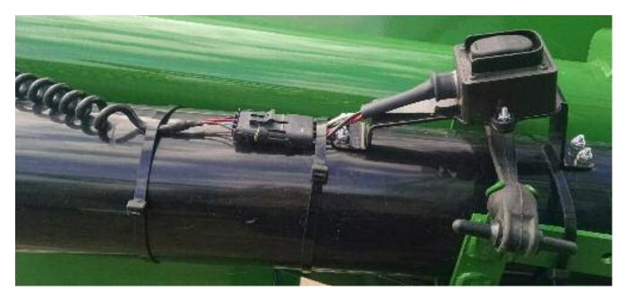
Plug in the coiled cable plug into the rocker switch plug. Use 2 heavy duty cable ties and fasten as shown in the picture. Place the rubber retainer under the formed handle and latch in place. This will retain the spout in the transport position.
