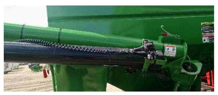
Go back to where the cable transitions from a straight cable to a coiled cable. Loop the coiled cable around the telescopic spout as shown in the picture.
