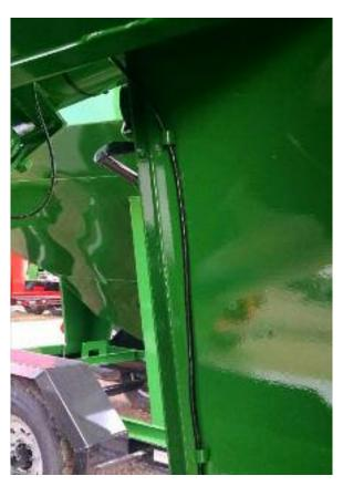
Locate the cable tabs on the inside of the front left leg of the seed tender. Transition the straight cable from the seed tender body to the seed tender leg.
