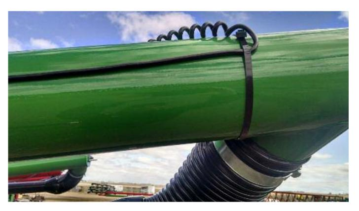
Locate the position on the cable where the coiled cable transitions to the straight cable. At this junction, attach the cable to the auger spout on the backside of the upper auger tube. Use a heavy duty cable tie and attach the cable as shown in the above picture. The straight cable should follow the auger tube towards the seed tender and the coiled cable should follow the telescopic spout.
