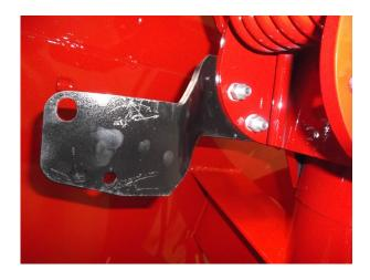
Step 3: Install the Lower Actuator Bracket. The first bracket will be installed next to the hopper body. The bracket should be installed so the bend is towards the centerline of the auger tube. Attach using 2 - 3/8" x 1-1/2" bolts, 2 - 3/8" Nuts, and 2 - 3/8" lock washers. Tighten all fasteners.
