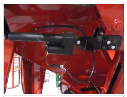
Step 8: Connect the weather pack connectors together. Leave some slack in the harness and route the harness along the side of the tender. Keep harness in place using wire ties.
