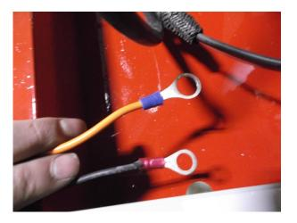
Step 10: Cut the eyelet connectors off of the positive and negative battery wires. Replace the positive fuse wire with a 3/8" eyelet connector (crimp in place) and replace the negative wire with a 5/16" eyelet connector (crimp in place).
