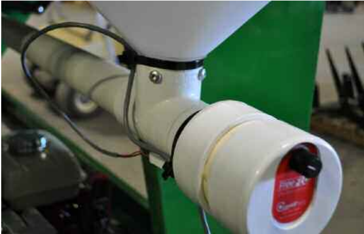
Zip tie wires to the inoculator
