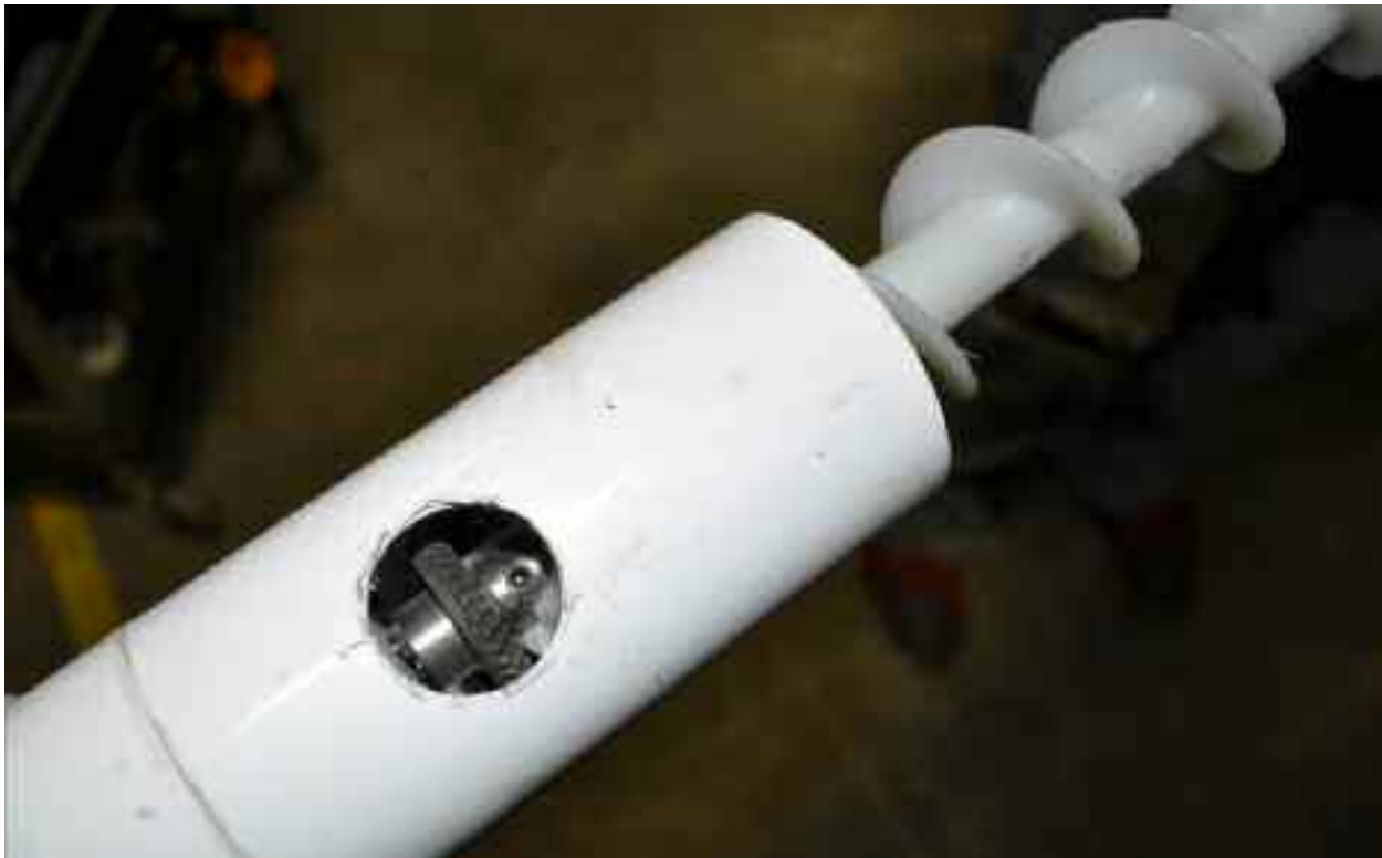
Mounting the auger to the inoculator Attach the auger to the motor using a set screw.
