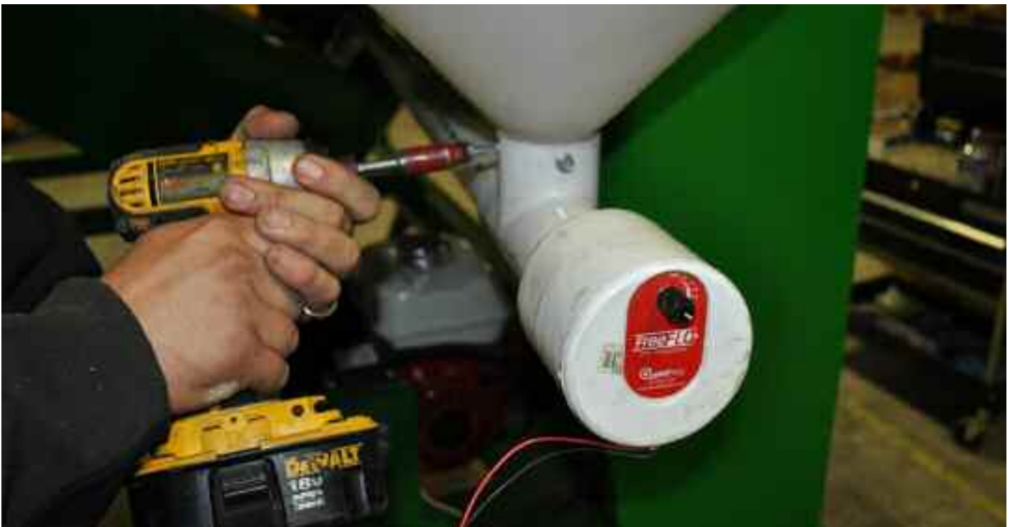
Attach the motor end of the auger to the inoculation tank with screws provided.
