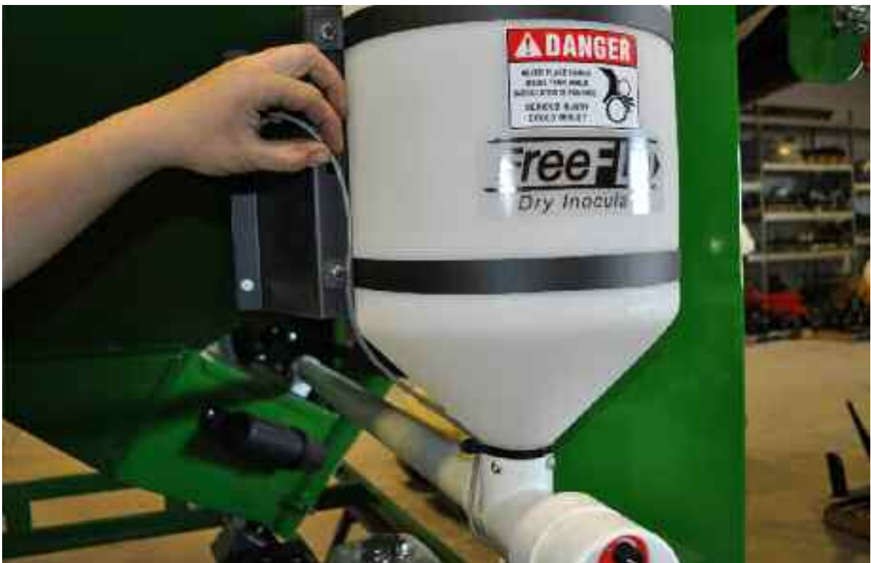
Drill a hole in the bracket and measure wire to be able to reach the hole. Mark the wire as a guide.
